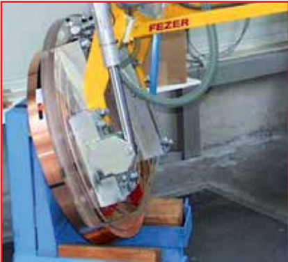
Flattened suction plate for engagement of upright coils with varying diameters
