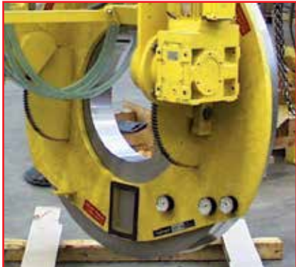
Look through: Suction plate with vision panel
