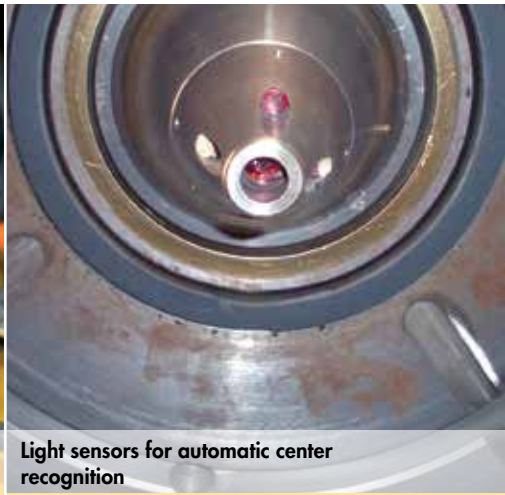
Light sensors for automatic center recognition
