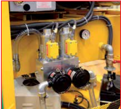
Single suction chamber control via impulse valve
