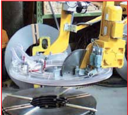
Look through: Suction plate in plexiglass design
