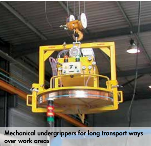
Mechanical undergrippers for long transport ways over work areas
